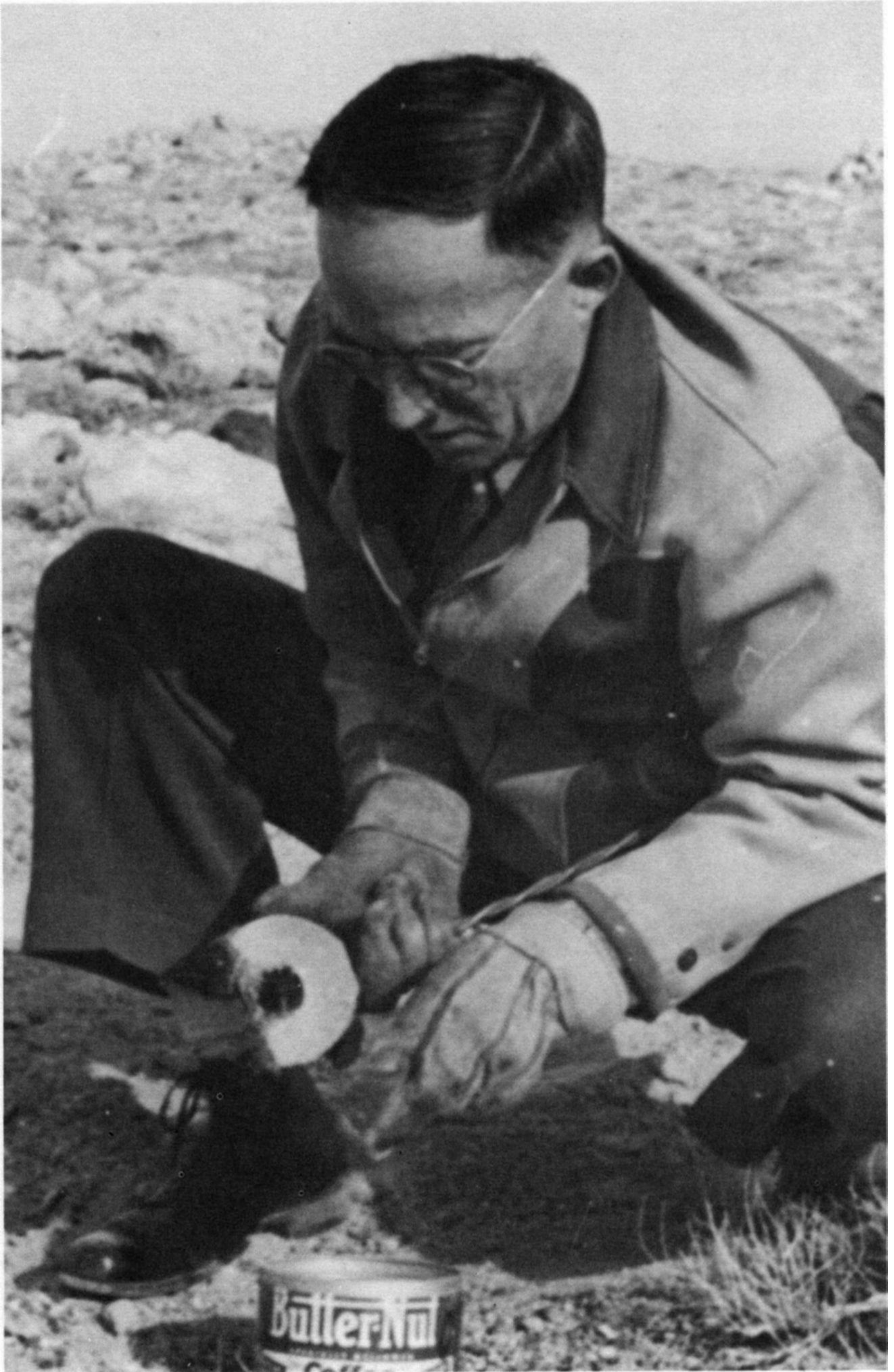
Dr. Ninger collecting magnetics on Crater rim. From these he separates the spheroids which are believed to be condensation products from the exploded meteorite.
